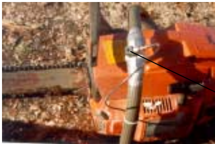
Figure 6 – Measurement of x-axis on the chainsaw – no intervention
